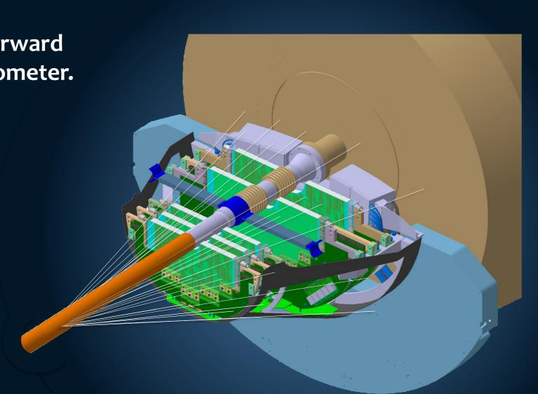
The hadron absorber prevents the MUON spectrometer from resolving the details of the vertex region. **The Muon Forward Tracker (MFT) will track the particles before they enter the hadron absorber**, by means of an assembly of silicon pixel planes → To be installed in 2020
