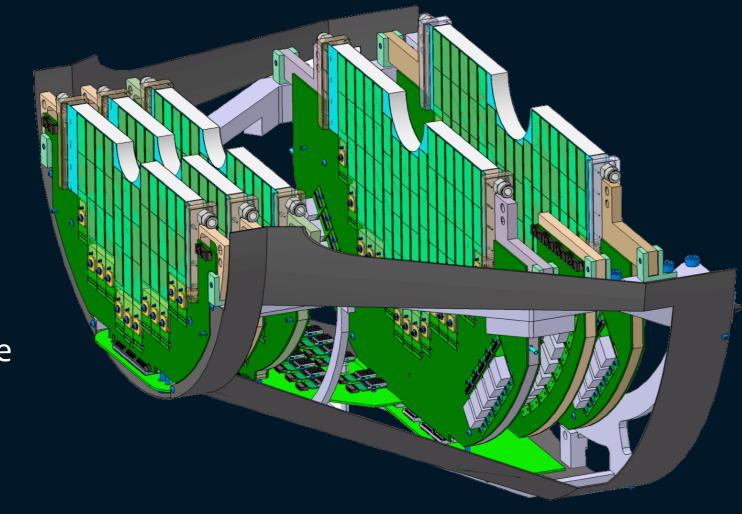
MFT water-cooling studies done through composite coldplate and composite ladder calculations assuming a consumption of 50 mW/cm² for sensors and 20 °C water flowing at 1 m/s:
