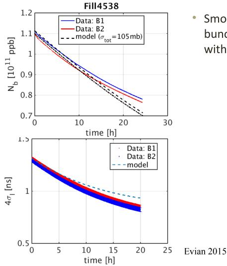
Smoother current decay and more bunch length damping is observed with respect to the model prediction
