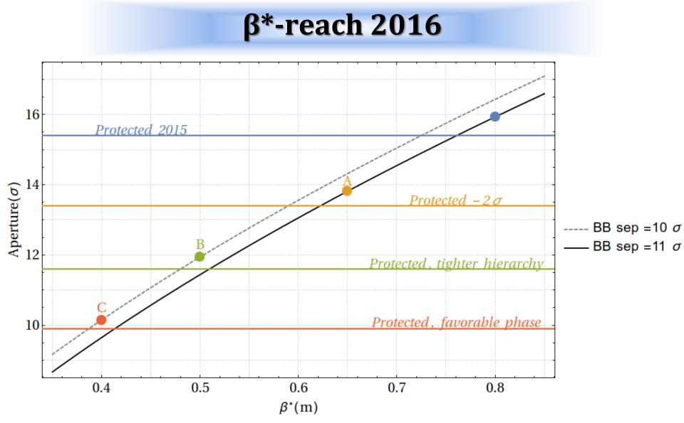
• With tighter hierarhcy in IR7/6,  $10\sigma$  BB separation, optics with re-matched phase, and assuming aperture does not deteriorate =>  $\beta^*$ =40 cm possible
