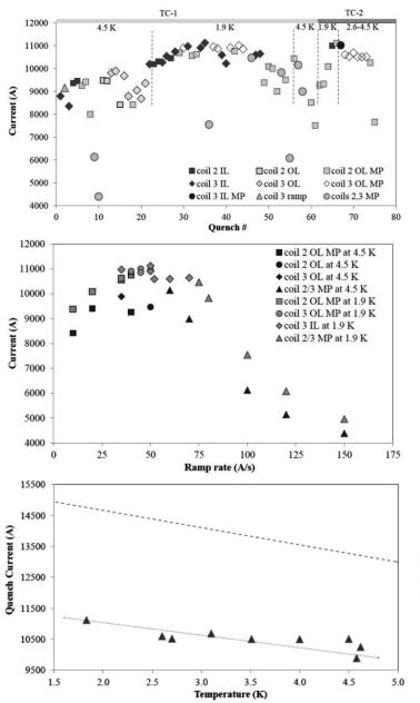
Most quenches at low ramp rates, all holding quenches and quenches at intermediate temperatures initiated in the mid-plane block of the outer coil layer
