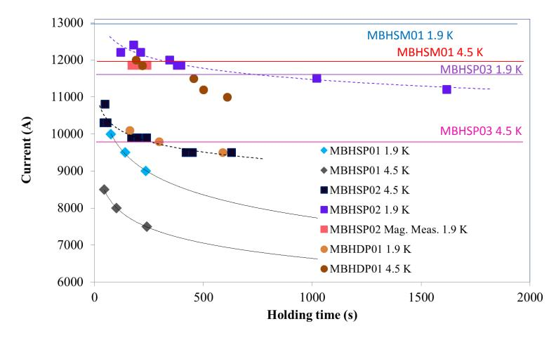
MBHSP01 shows steeper dependence on time but the type of dependence is similar (trendlines are logarithmic functions)
