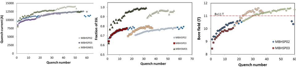
The improved quench performance of coil #8 (wrt #5 and #7 in MBHSP02 with similar design and fabrication process) in the dipole mirror structure suggested that the large mid-plane shim was likely a major cause of the conductor degradation in the dipole model MBHSP02
