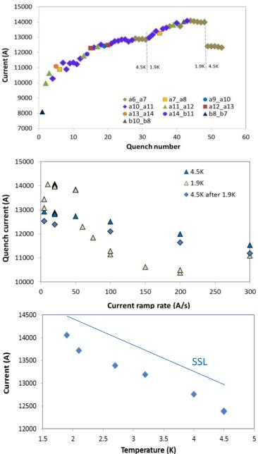
The goal of this test was to understand the role of coil design and (reduced) pre-stress on its quench performance
