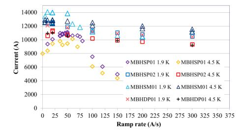
Quenches happen in "usual" locations (similar to training) with an exception at lowest ramp rate: for magnets which failed holding current tests, when a reverse dependence is observed quenches develop in the mid-plane segment in the OL 19
