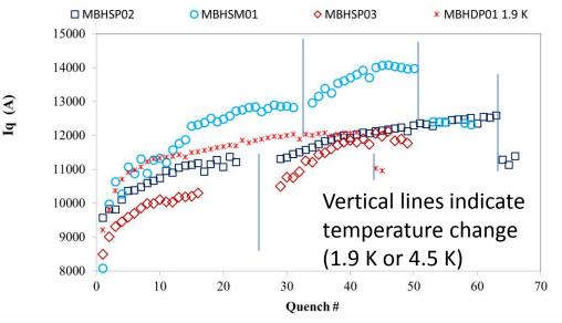
During training the absolute quench current does not depend on the temperature (1.9-4.5 K)
