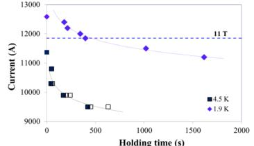
all the holding quenches started in the outer-layer mid-plane block of coil 7
