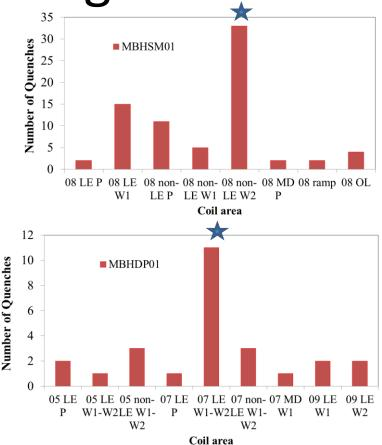
Most quenches develop in the non-straight sections around the first wedge (and the pole) or often asymmetrically around the second wedge (non-LE).
