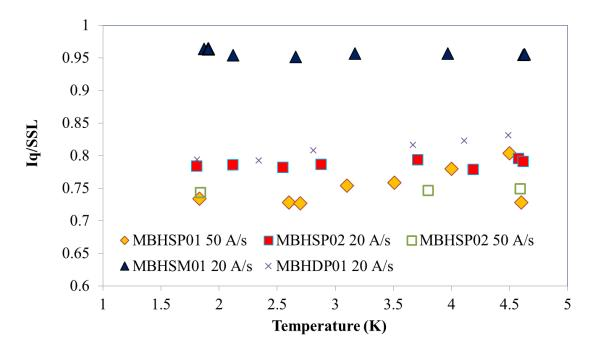
Quench locations follow the pattern in training quenches. Worth mentioning : At the end of the training of MBHSP02, quenches at 4.5 K developed in the OL of coil 07 the same location for quenches above 3 K.
