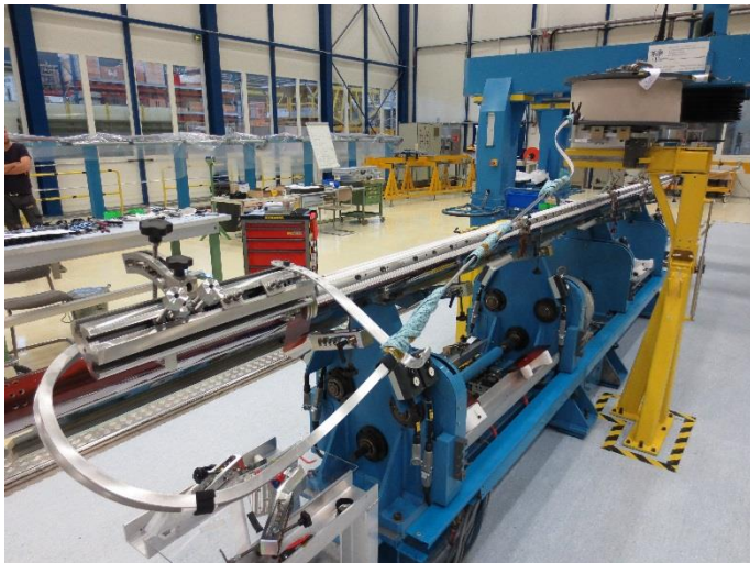
3 rd coil, with braided Sc cable during winding
