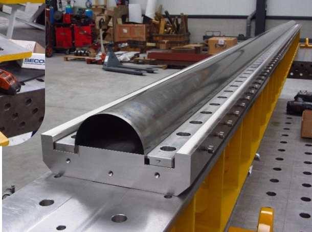
6 m long impregnation fixture
