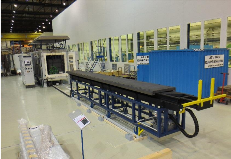
6.5 m long reaction furnace – fully operational
