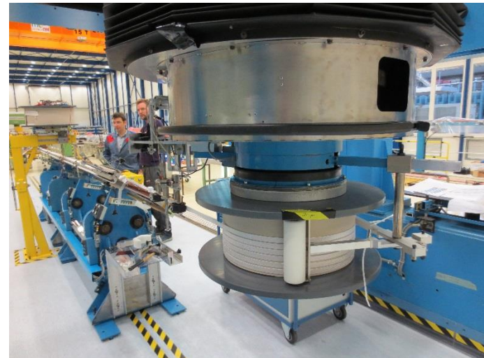
New clutch / PCS for better control of the tension on cable during winding
