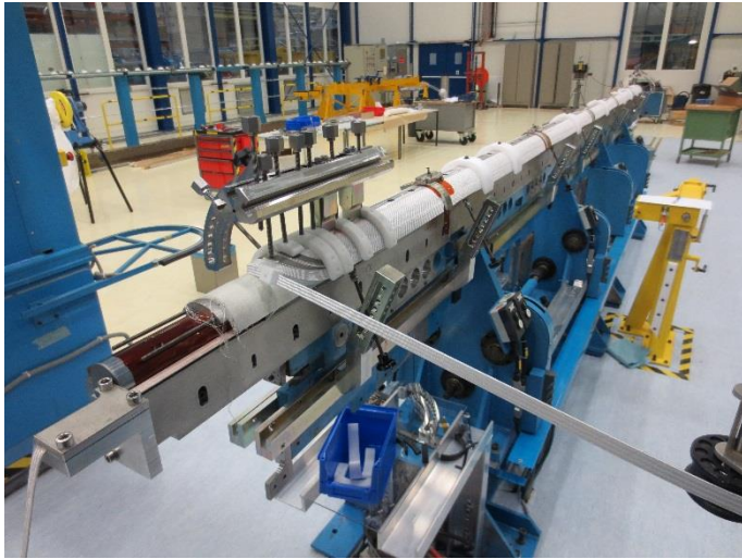
2 nd coil with braided Cu cable during winding
