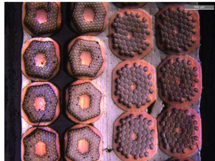
Figure 12. Image of the lower layer splice of the coil SMC 11T #2.
