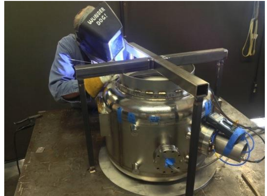
Large fixtures needed to control warping
