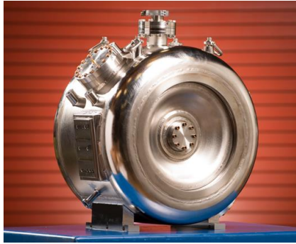
Jacketed SSR1 cavities (4 Type-A, 4 Type-B)
