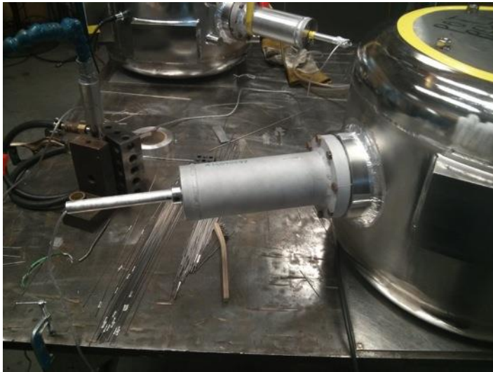
Thermal cameras insertion tubes (above)
