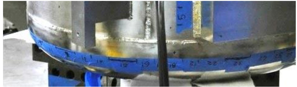
Welding inch-by-inch on 6 mm thick steel
