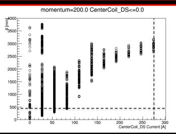
Flip mode optical functions at the absorber as a function of current in the centre coil. 140 MeV/c (left); 200 MeV/c (right). 4 T in the tracker requires 274 A.
