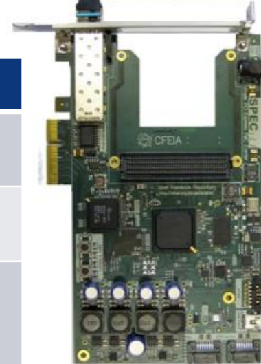
FMC mezzanine board, to be plugged on the PCIe carrier (SPEC)
