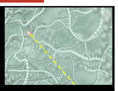
The highly ionizing particle leaves a cylindrical trail of damage in the plastic track etch detectors
