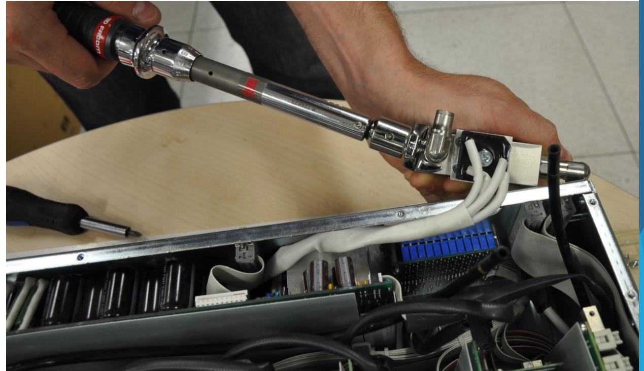
Screw new connector with the right torque (dynamometric Key)
