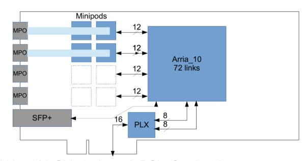
output bandwidth ~100 Gbits/s through PCle Gen3 x16
