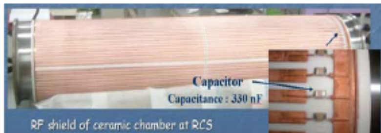
RF shielded ceramic pipe for RCS Courtesy YH. Chin, J-PARC
