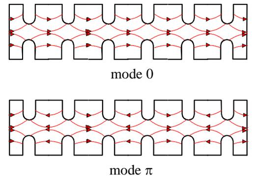
Mechanical errors → differences in frequency between cells → to respect the new boundary conditions the electric field will be a linear combination of all modes, with weight
