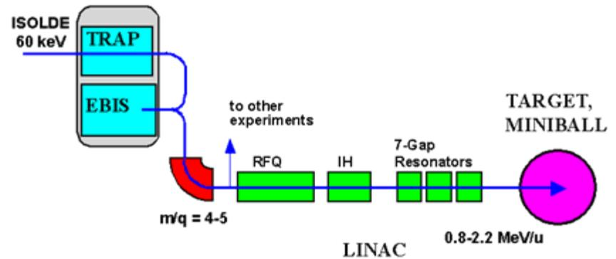
The REX heavy-ion post accelerators at CERN. It is made of 5 short standing wave accelerating structures at 100 MHz, spaced by focusing elements.
