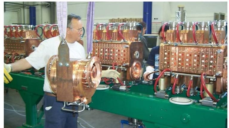
$\pi/2$ -mode in a coupled-cell structure
