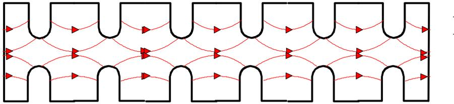
To obtain an accelerating structure for protons we close our disc-loaded structure at both ends with metallic walls  $\rightarrow$  multiple reflections of the waves.
