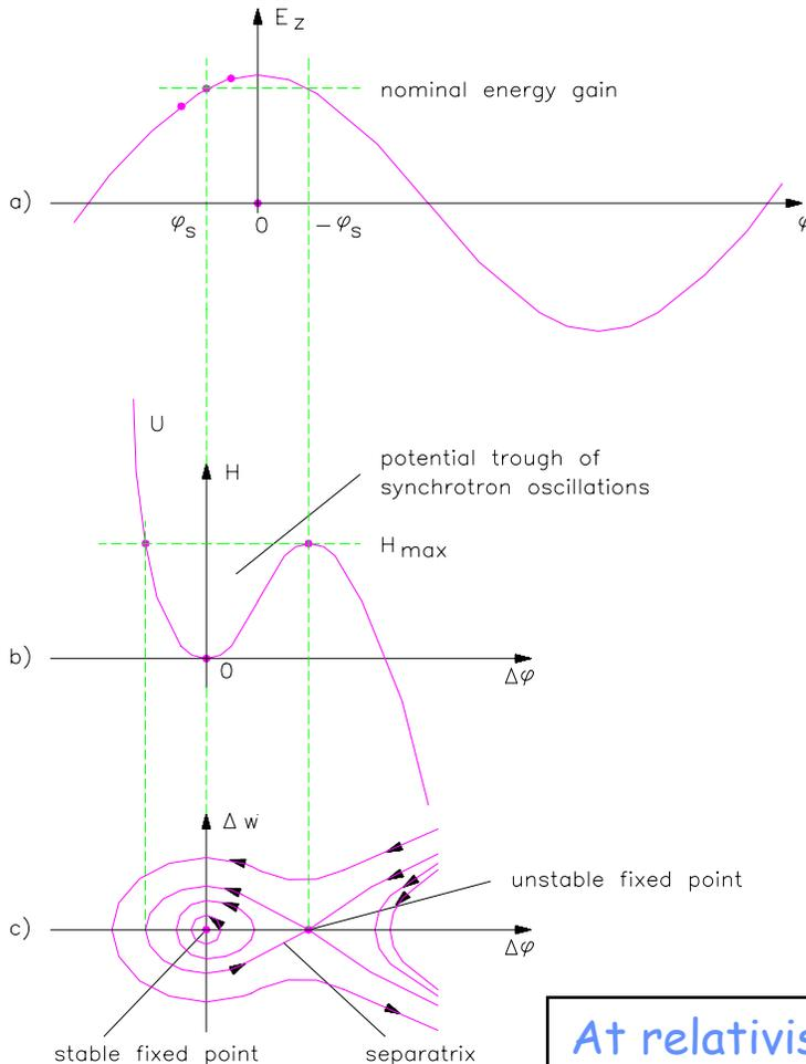
→ Ions are accelerated around a (negative = linac definition) synchronous phase.
