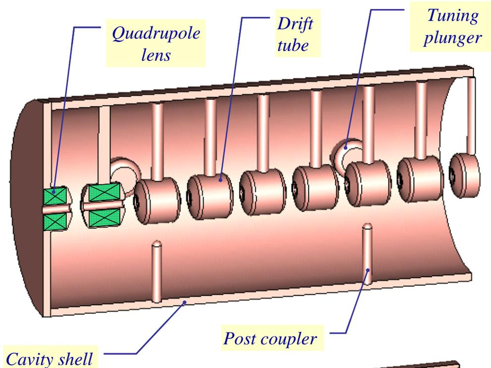
Standing wave linac structure for protons and ions,  $\beta=0.1-0.5$ ,  $f=20-400$  MHz
