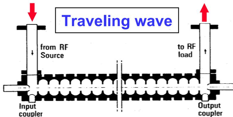
Chain of coupled cells in TW mode
