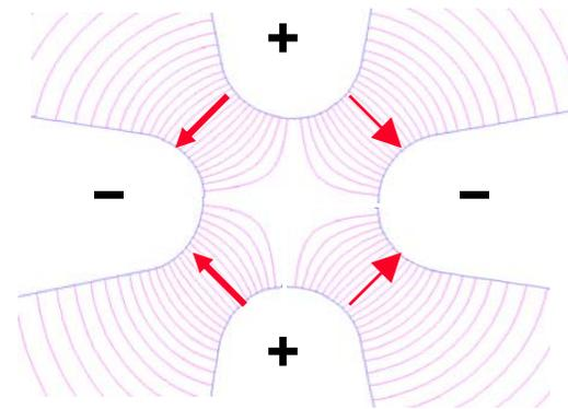
2. The vanes have a longitudinal modulation with period =  $\beta\lambda$  → this creates a longitudinal component of the electric field. The modulation corresponds exactly to a series of RF gaps and can provide acceleration.
