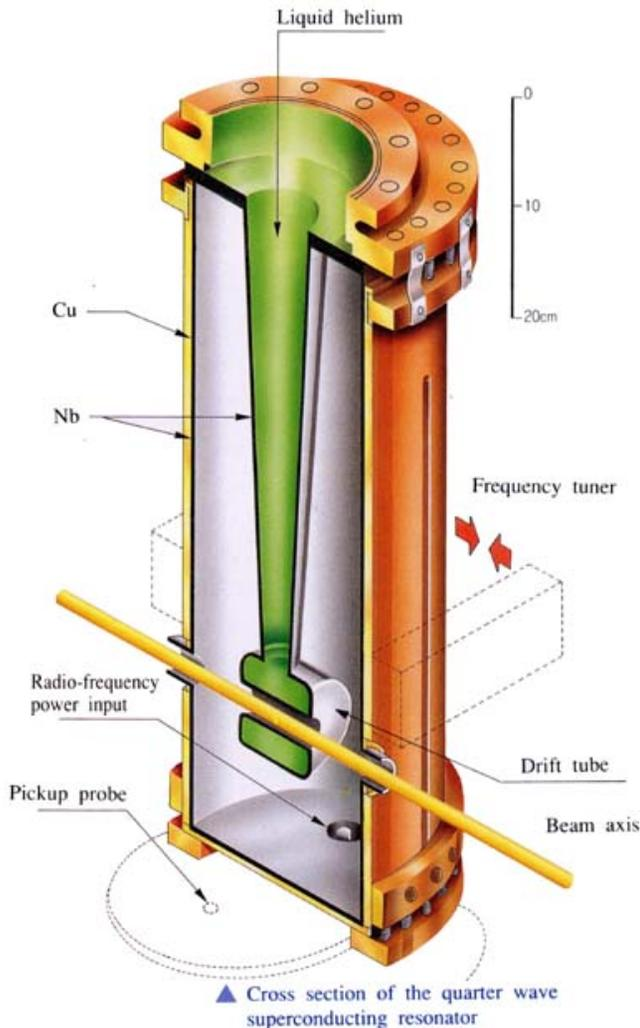
Simple 2-gap cavities commonly used in their superconducting version (lead, niobium, sputtered niobium) for low beta protons or ion linacs, where  $\sim$ CW operation is required.
