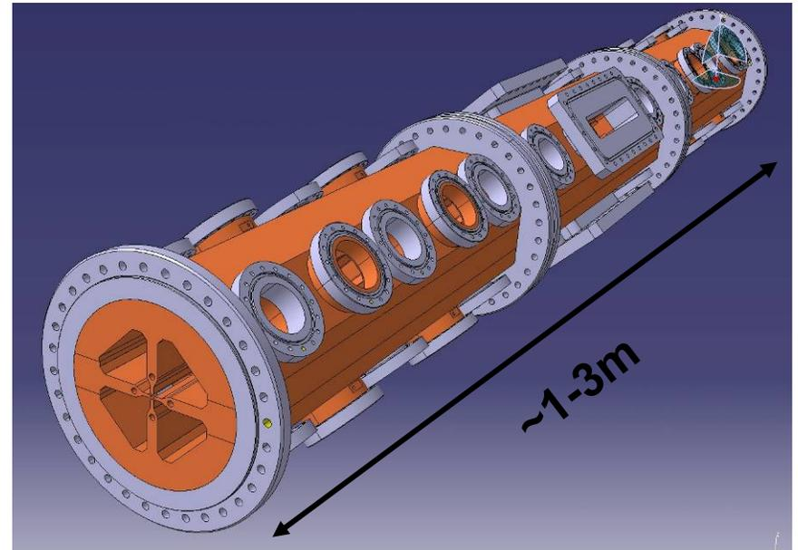
RFQ = Electric quadrupole focusing channel + bunching + acceleration
