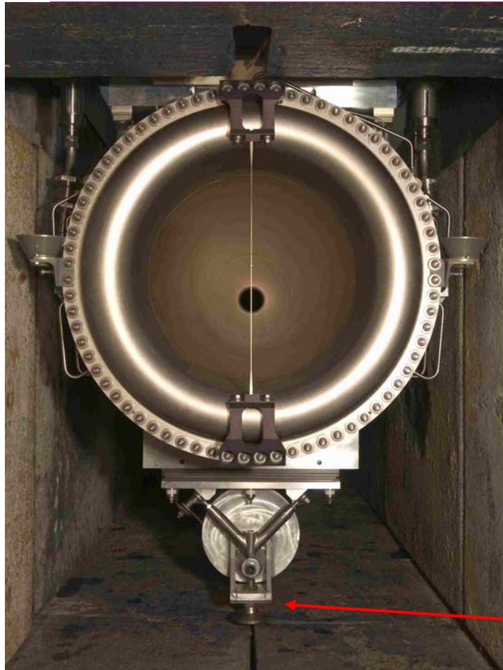
Horn 2 before beam 1.5 inch clearance foot to floor
