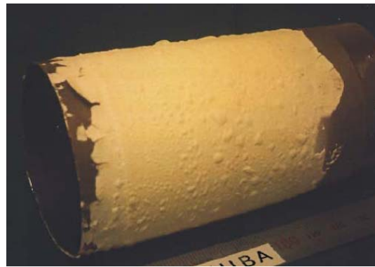
Ceramic w/ Al 2 O 3 based sealing falls off the Ti-Alloy tube (400°C 1hour), while test piece without sealing is not damaged (600 ° C 2hour).
