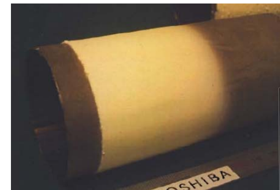
Ceramic w/ Al 2 O 3 based sealing falls off the Ti-Alloy tube (400°C 1hour), while test piece without sealing is not damaged (600 ° C 2hour).
