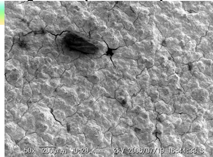
Sealing w/ Al 2 O 3 -based mat.(×50)
