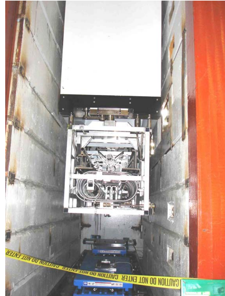
Target on module, ready to crane into beam
