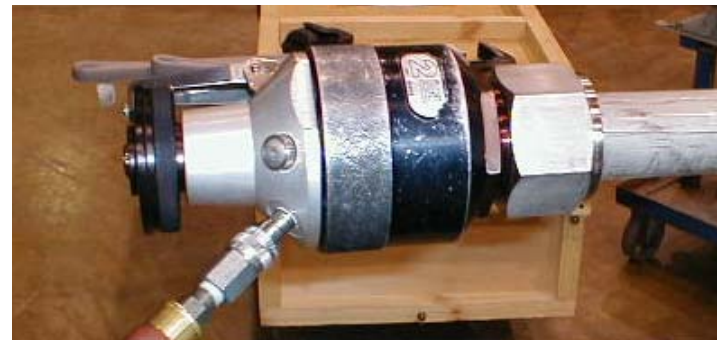
Hydraulic Swaging of compression fitting
