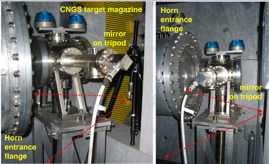
NBI–2006 Workshop, CERN, Sept. 06<sup>th</sup>, 2006, Page 4 CNGS Horn & Reflector Vibration-Measurement in TCC4
