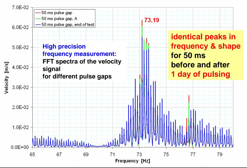
NBI–2006 Workshop, CERN, Sept. 06<sup>th</sup>, 2006, Page 27 CNGS Horn & Reflector Vibration-Measurement in TCC4
