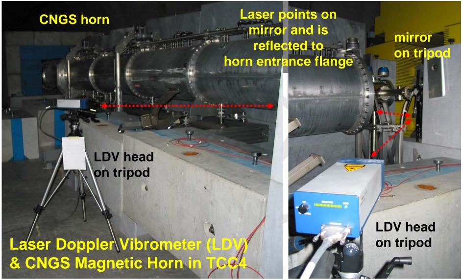
NBI–2006 Workshop, CERN, Sept. 06<sup>th</sup>, 2006, Page 3 CNGS Horn & Reflector Vibration-Measurement in TCC4
