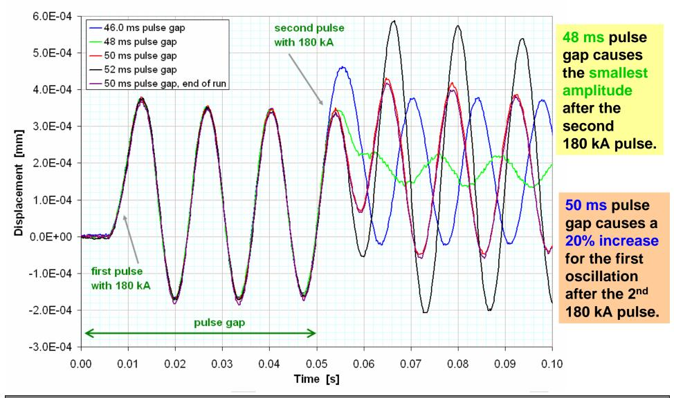
NBI–2006 Workshop, CERN, Sept. 06<sup>th</sup>, 2006, Page 21 CNGS Horn & Reflector Vibration-Measurement in TCC4
