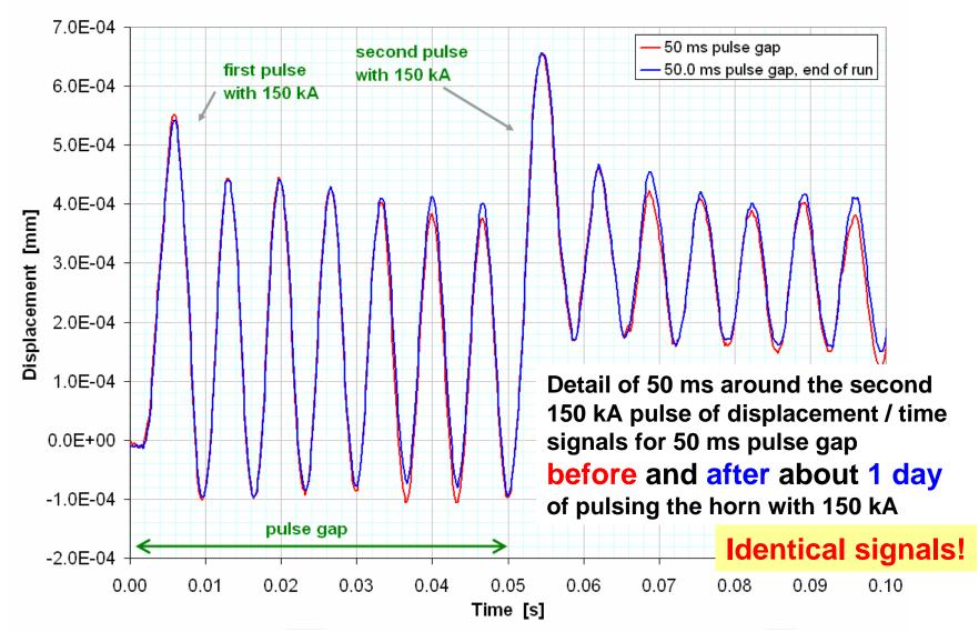
NBI–2006 Workshop, CERN, Sept. 06<sup>th</sup>, 2006, Page 10 CNGS Horn & Reflector Vibration-Measurement in TCC4
