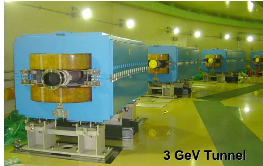
Kicker & Septum Magnets for fast extraction
