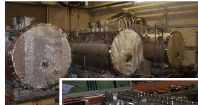
Kicker & Septum Magnets for fast extraction
