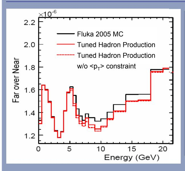
• F/N does not change in focusing peak by this procedure Changes in high energy tail ~10%, but stable to 2%
