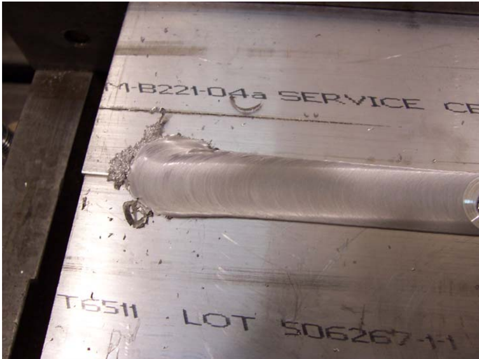
Entry point of FSW tool on test weld
