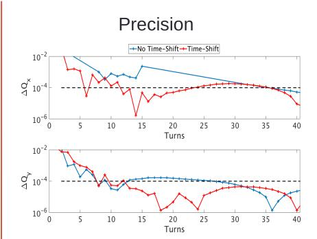
Precision below 10<sup>-3</sup> in less than 10 turns for both planes
