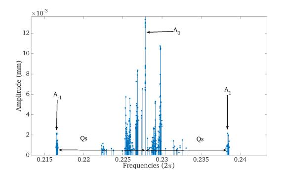
Results from ANKA ring using a sliding window to compute sidebands and the synchrotron tune and applying the formula for the RMS energy spread
