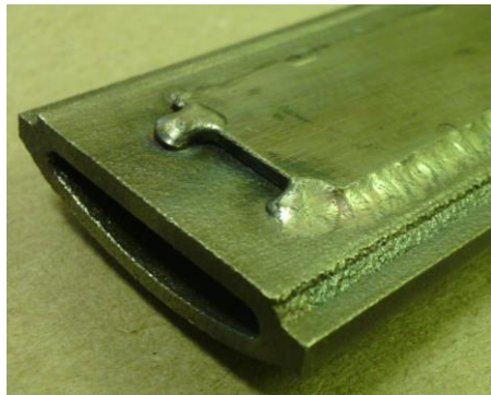
3D printed cooling channel
