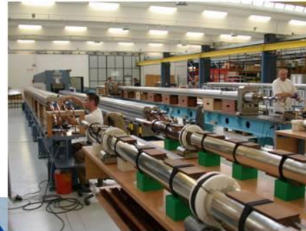
Assembly of 15 m long coils in industry, 2003
