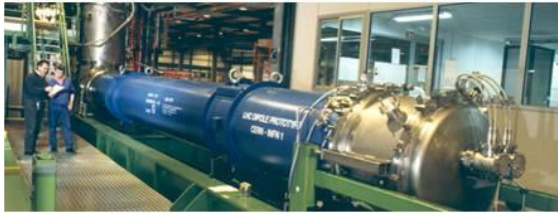
First LHC dipole prototype on the test bench (June 1994)
