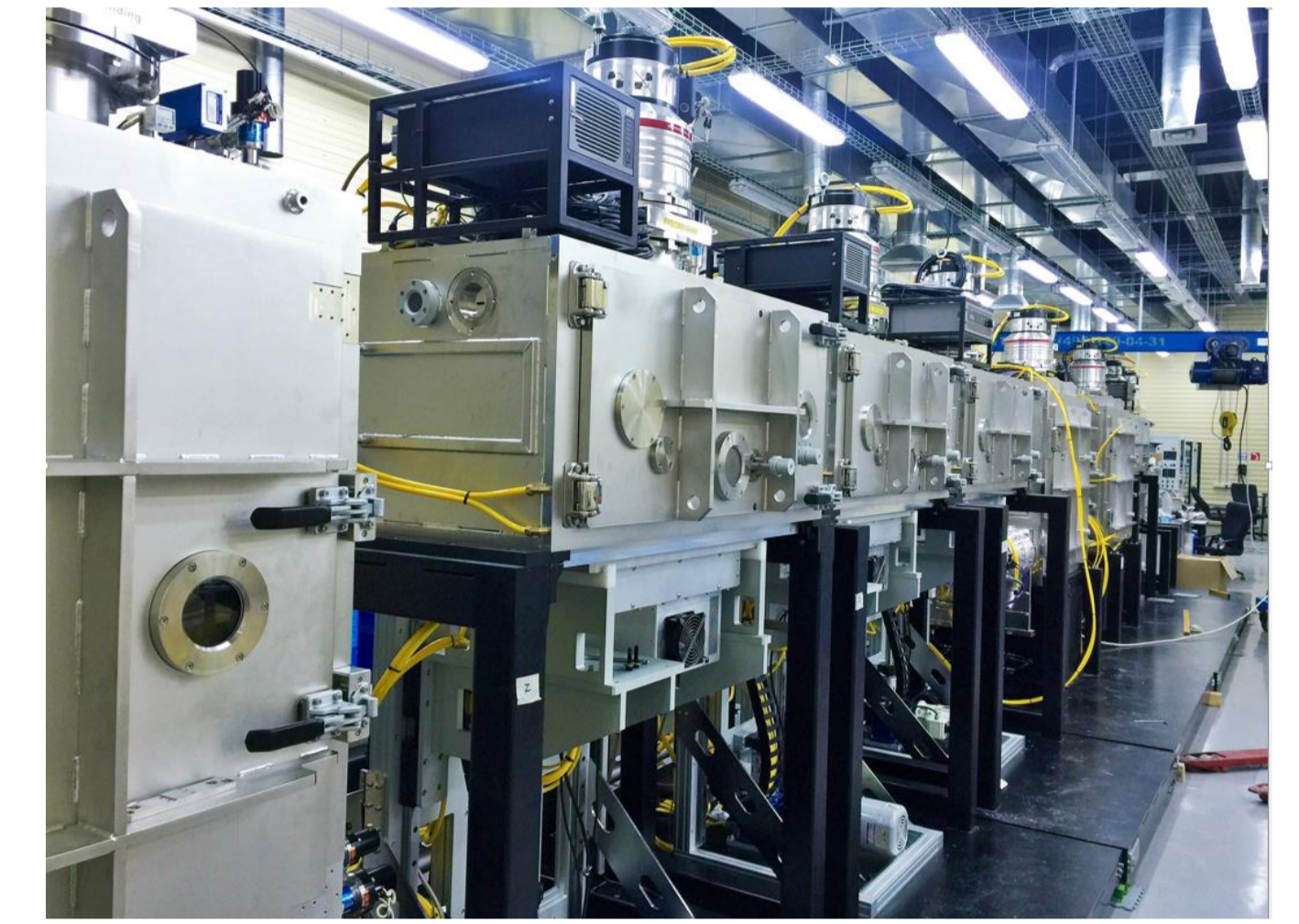
New buffer layer deposition line commissioned in Moscow PLD-HTS system to be commissioned by the end of 2016
