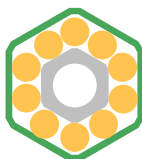
Coil without G11 structure → more engineering current density
