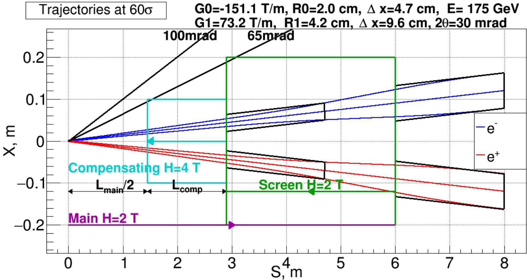
Compensating solenoid  $R = 0.1 \text{ m}$ , screening solenoid  $R = 0.2 \text{ m}$ .
