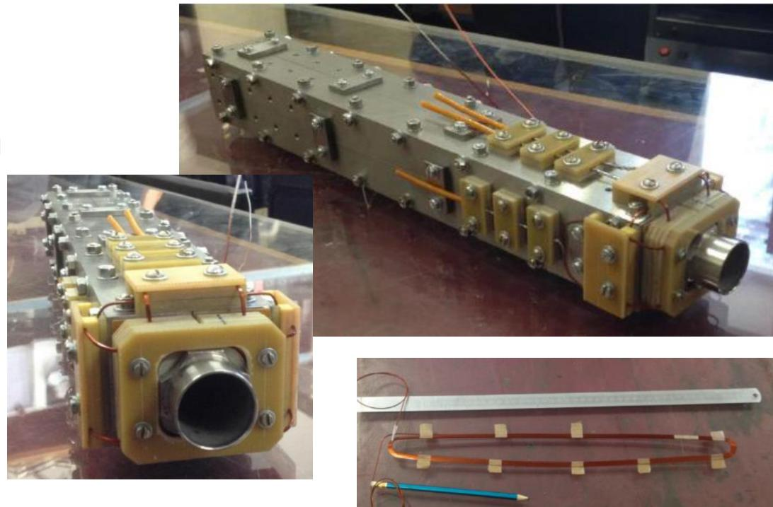
During the first cryo-test (01.02.16) the current of 1060 A was achieved after 3 quenches.
