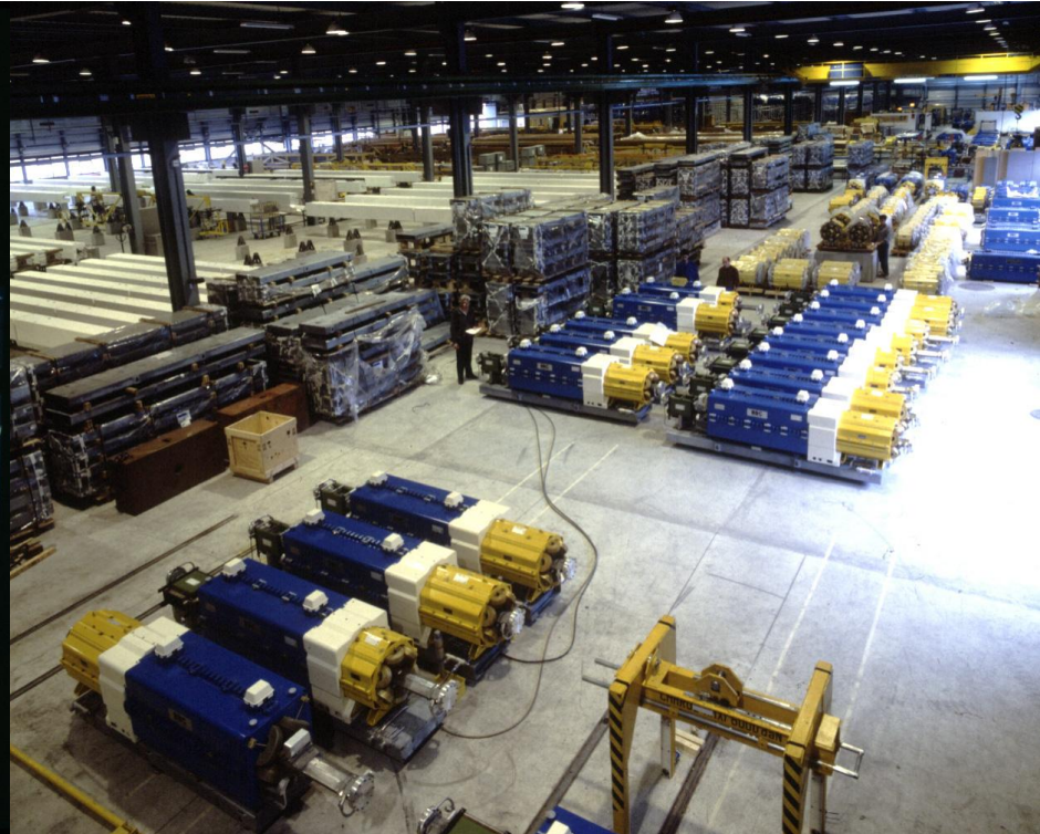
Hall full of LEP magnets waiting to be installed in November 1987
