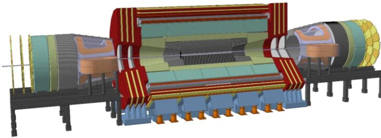
**Partially shielded solenoid with dipoles**
