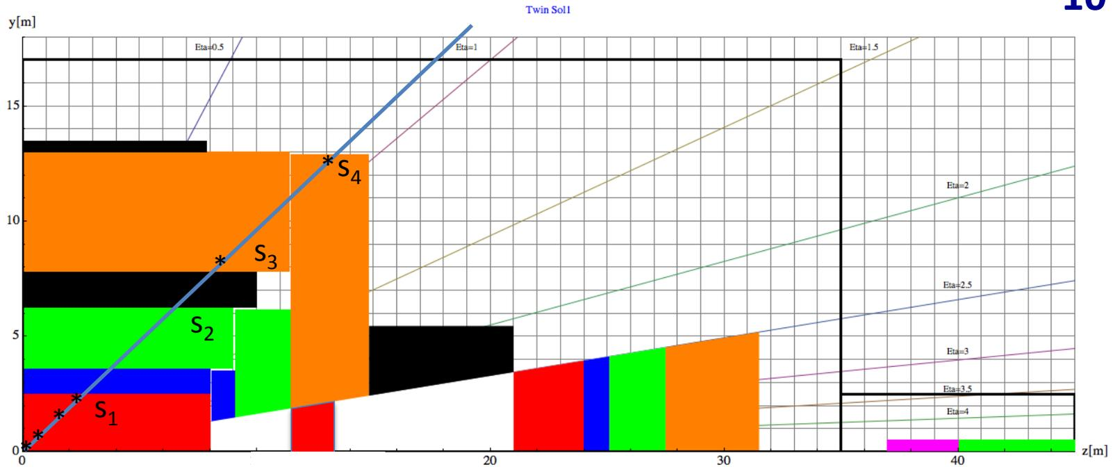
Fit of the template function to 14 measurement points of 23 $\mu$ m in the inner tracker and 1 layer in the muon system with a resolution that is much better than the multiple scattering limit.
