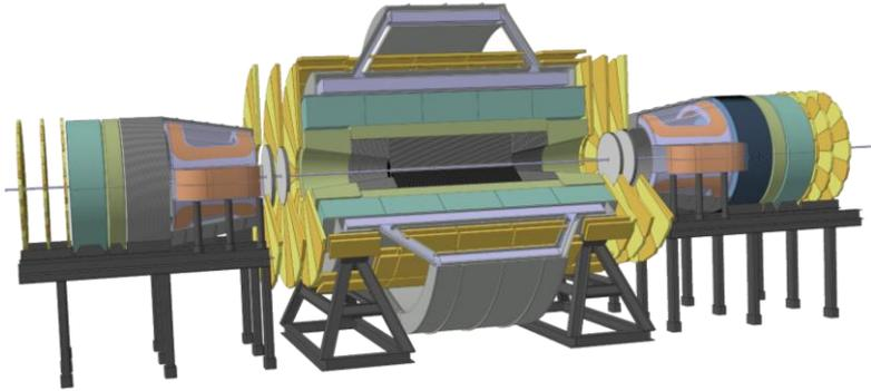
**Twin solenoid with dipoles**
