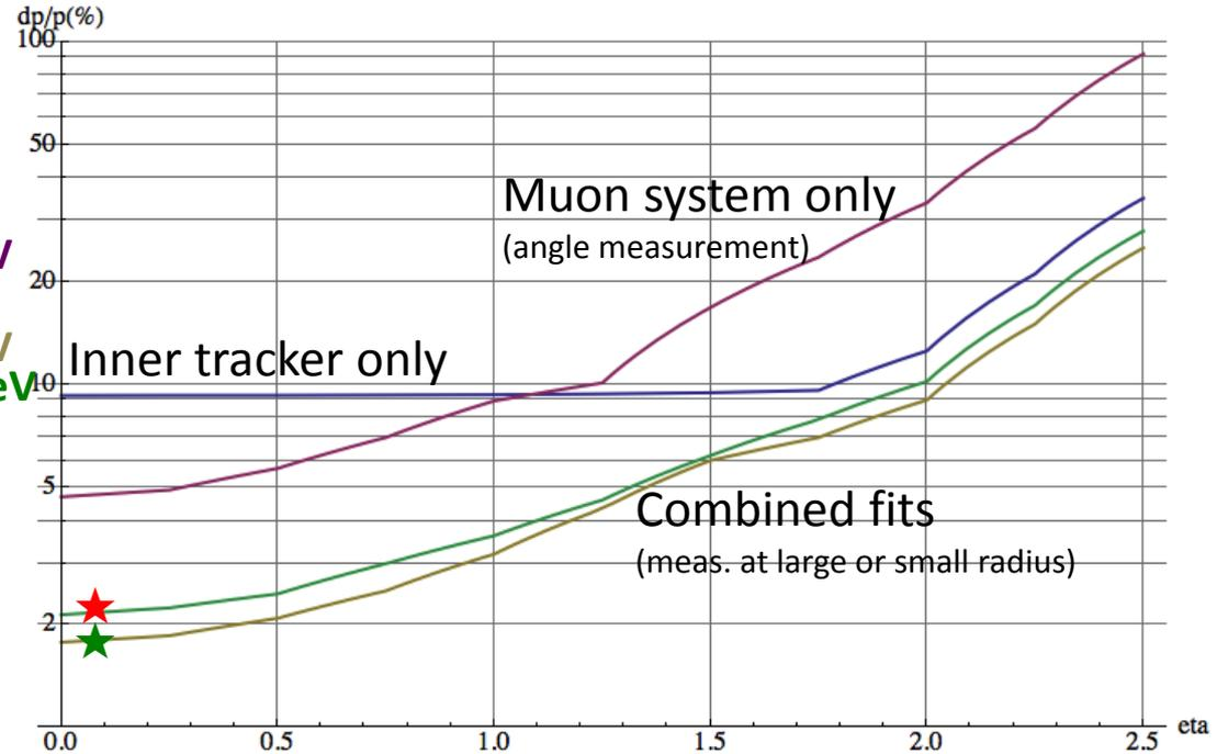
**Twin Solenoid assuming inner tracker with baseline resolution curves and multiple scattering limit in the muons system.**
