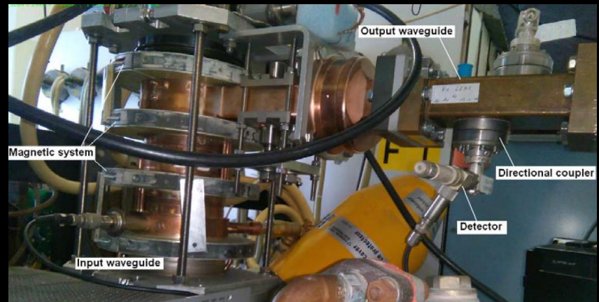
The rear view of the test set-up
