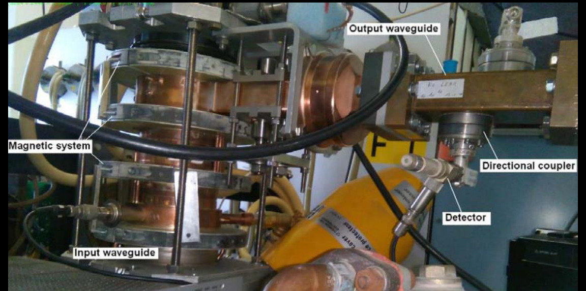
The rear view of the test set-up
