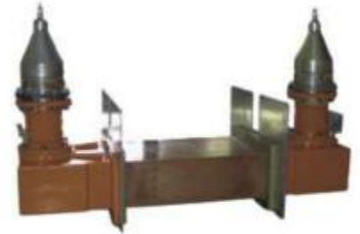
Figure 4: Setup to measure the prototypes of both proposed RF loads.
