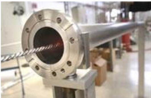
NEG (Non-Evaporable Getter) TiZrV thin film coatings Technology used to create and maintain ultra-high vacuum in the accelerator vacuum chambers
