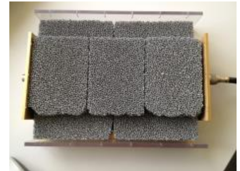
Broadband microwave measurement of SiC foam
