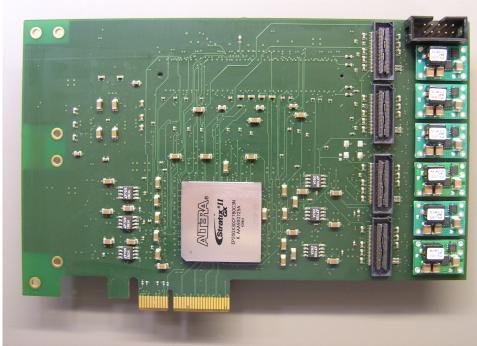
Optical IN: 4 x 16 bit @ 75-156 MHz (1.2-2.5 gbit/s) Copper IN: 2-4 x 48 bit @ 66-133 MHz (3.1-6.3 gbit/s) depending on cable length o OUT: PCI-E 4 x 16 bit @ 125 MHz (2.0 Gbit/s)
