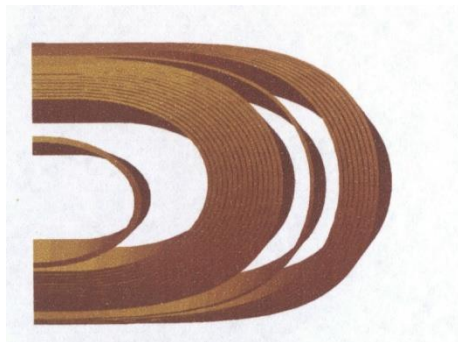
End of a \cos\theta coil [S. Russenschuck, World Scientific, Fig. 32.13]
