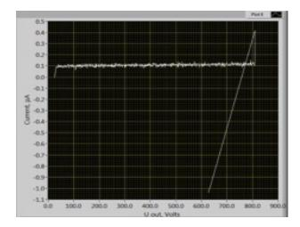
Coil to structure Failure occurred with no "pre-cursor"
