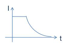
By evaluating the MIITs from the current decay, we obtain an estimate of the hot spot temperature  $T_{\text{max}}$
