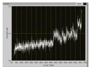
Coil to protection heater Steep current rise is another "precursor" of failure
