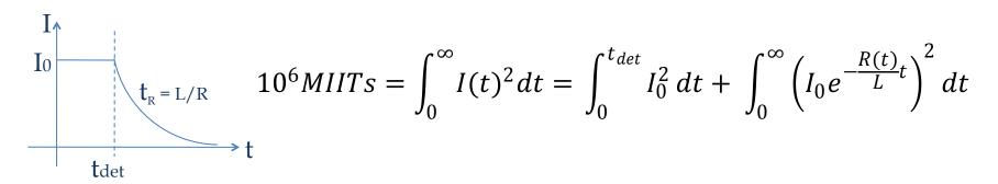
By assuming that the resistance is constant over time, we can obtain a estimate of what is the required resistance
