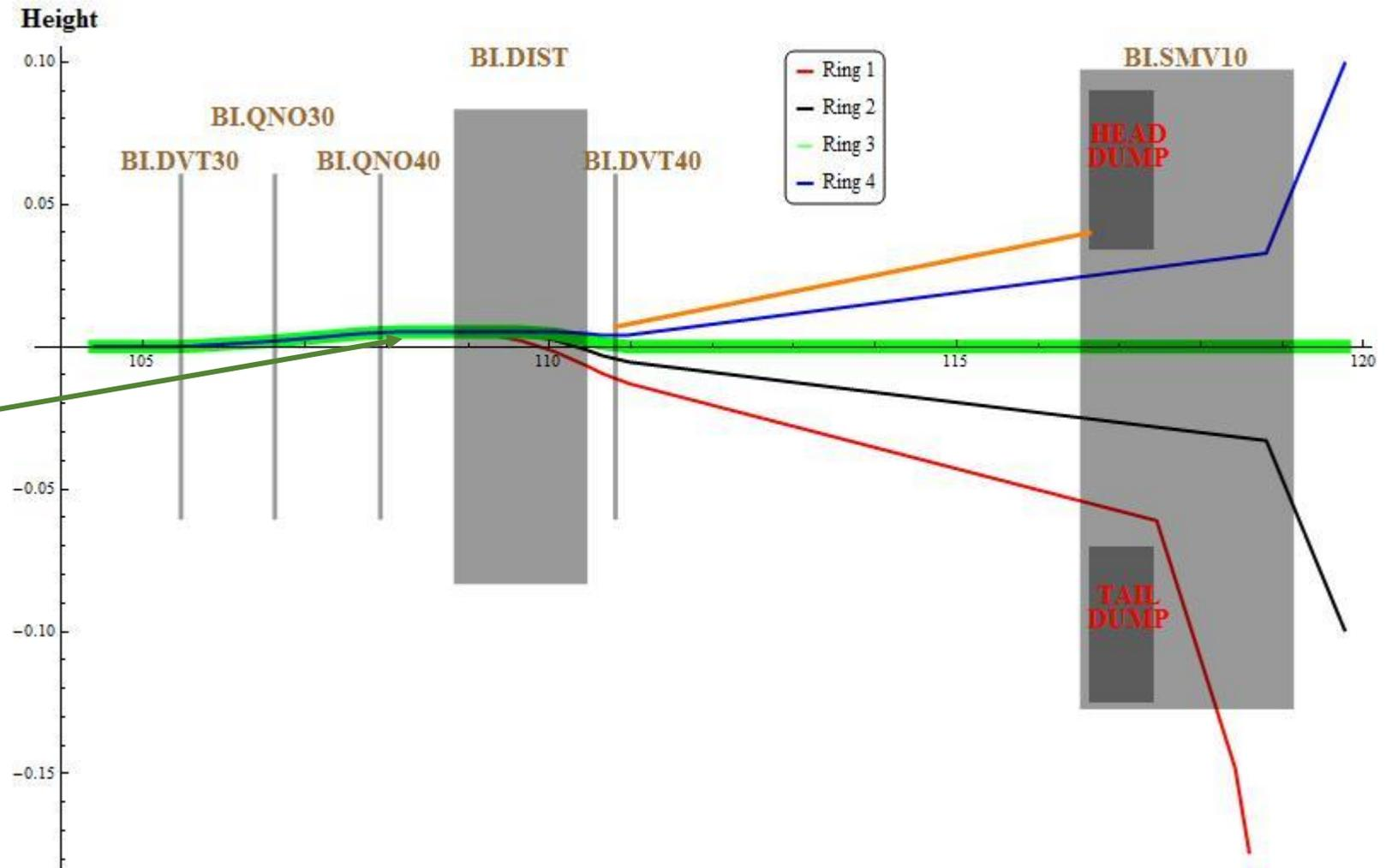
Only the middle part of the pulse from LINAC2 is used. The head and tail of the pulse are dumped
