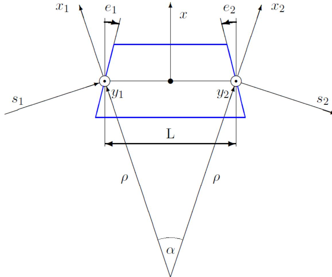
If the pole face angles of the DIST/SMV10/BVT10 are not accurate, then the effect will be felt essentially only in the vertical plane.
