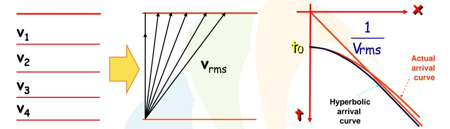
• It replaces the layered medium by a constant effective velocity ( $V_{RMS}$ ) that fits the short spread moveout (x<z).
