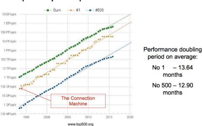
Large HPCs use a variety of architecture Half of computational power is concentrated in a small number of machines; Small HPCs use x86 architectures. Typically, these are ordinary server racks, with Infiniband interconnects. 94% of the bottom 400 of the Top 500 (including the last 130) are all x86
