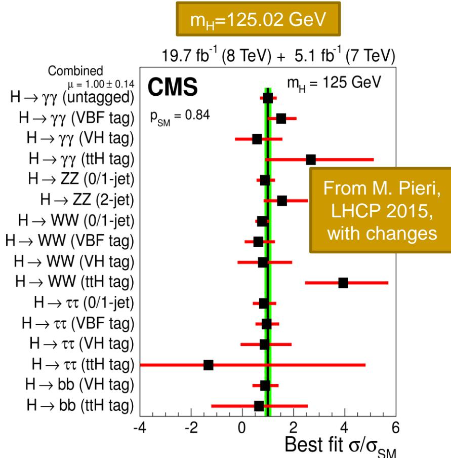
$$\mu = 1.00 \pm 0.09(\text{stat.}) \pm 0.07(\text{syst.}) \pm 0.08(\text{th.})$$
