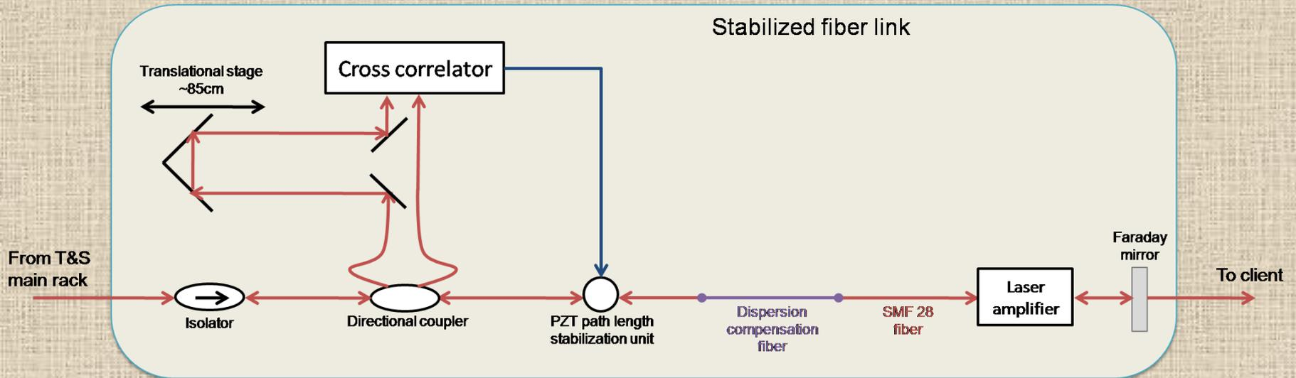
**Active stabilized links** are based on high resolution **round trip time measurements** and **path length correction** to stick at some stable reference value.
