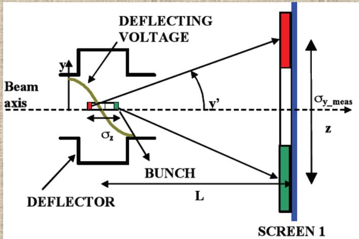
The beam is *streaked* by a *transverse RF cavity* on a *screen*. The image is captured by a camera. Longitudinal charge distribution and centroid position can be measured.
