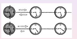
$$t_R = \frac{t_0 + t_A}{2} + \frac{k_{\epsilon}x}{c} = t_R^{(s)} + \frac{k_{\epsilon}x}{c}$$
