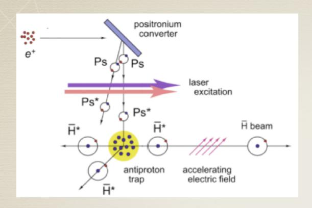
Positrons incoming from a  $\beta$ + hit a silicon microporous target, where they capture an electron and Positronium (Ps) is created.
