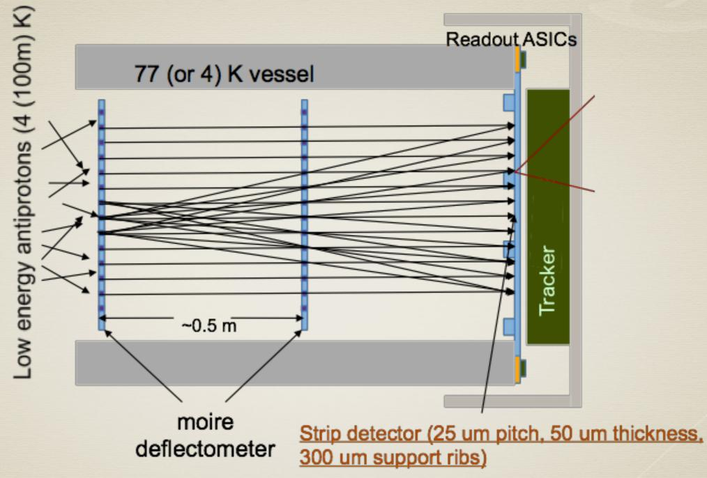
Detection of anti hydrogen through a hybrid detector:
