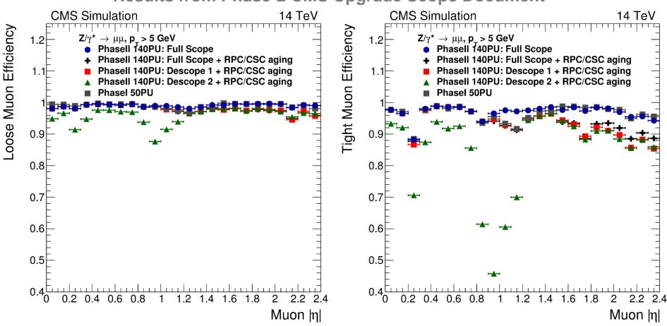
Loose Muon identification efficiency (left) and Tight Muon Identification efficiency (right) in Drell-Yan events as a function of the  $|\eta|$  of the simulated muon for different detector scenarios
