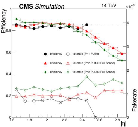
Electron identification in the endcap calorimeter for Drell-Yan events (left) and photon selection efficiency and fake rate in bins of  $|\eta|$  for samples of simulated events with a photon and a jet (right). Results are shown for reference configuration at <PU>=140 (red) and <PU>=200 (green) and Phase I configuration at <PU>=50 (black)
