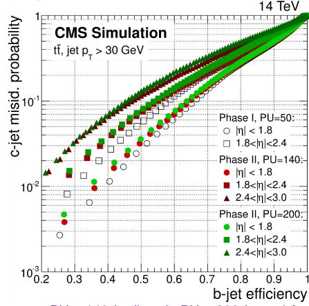
b-jet tagging performance studied with top-pair events at <PU>=140 (red) and <PU>=200 (green) for different pseudorapidity ranges. Results based on Phase I detector at <PU>=50 (open black) are also shown. Performance is expressed as misidentification probability for udsg-jets (left) and c-jets (right) as a function of b-jet tagging efficiency. Events are selected only if the correct primary interaction vertex is reconstructed. Good b-jet tagging capability extends to high pseudorapidity
