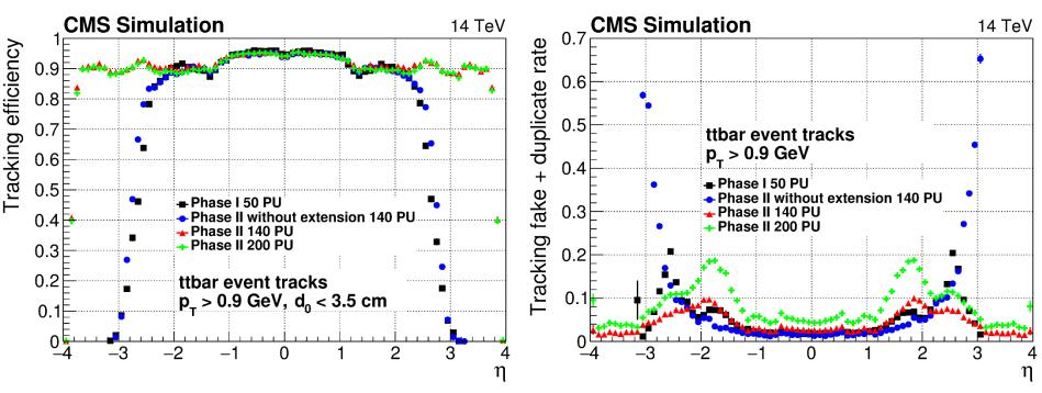
Track reconstruction efficiency (left) and track mis-reconstruction rate (right) for  $p_T>0.9 \, \text{GeV}$ , as a function of  $\eta$  for top-pair events. The results are shown for three configurations, the full scope detector with 140 (red) and 200 (green) pileup events and without the forward extension of the tracker (blue) with 140 pileup events. Results based on Phase I detector with 50 (black) pileup events are also included
