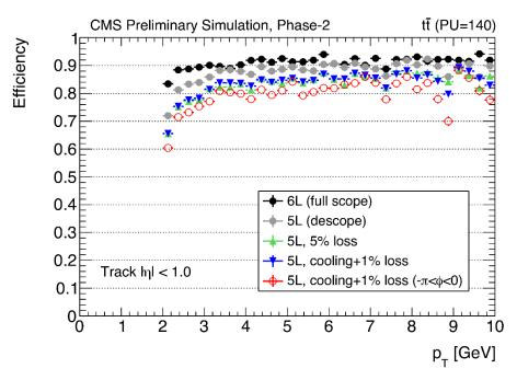
Track trigger efficiency as function of pseudo-rapidity and transverse momentum for different detector configurations, with top-pair charged particles. The red dots show the efficiency in the limited angular region of the missing cooling loop
