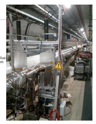
five stations: three backwards, two forward detectors: four plastic scintillator plates,
