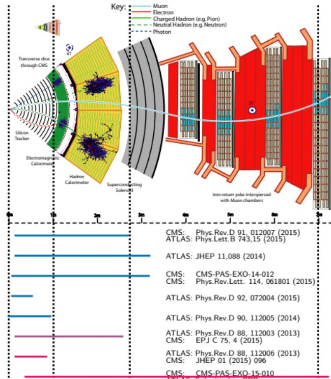
Exploit heaviness of new particles using  $dE/dx$
