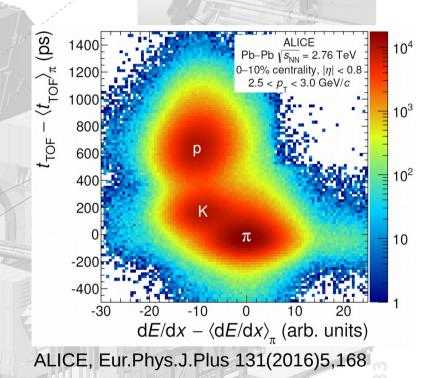
Combined *dE/dx* and TOF measurements offer π/K/p separation up to high momenta
