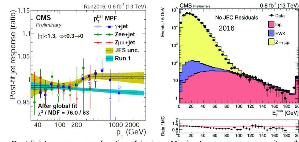
Post-fit jet response as a function of the jet transverse momentum. Same trend observed as in 2015 data, attributed to the change in local reconstruction in the HCAL. Missing transverse energy quite well modelled taking into account that residual jet energy corrections are not applied
