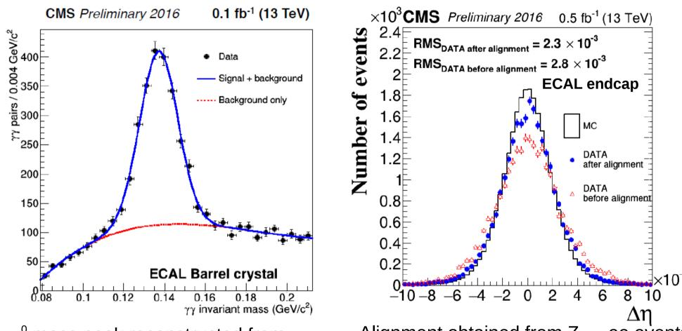
$\pi^{0}$  mass peak reconstructed from photon pairs in a single ECAL crystal  $\rightarrow$  used for intercalibration of ECAL crystal energies, RMS on relative energy scale during a fill is around 7% when this calibration is applied Alignment obtained from  $Z \rightarrow ee$  events In the ECAL barrel the RMS is roughly half compared to the endcaps
