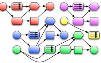
Run3 multi-threaded reconstruction cartoon: Colours represent different events, shapes different algorithms; all one process running multiple threads
