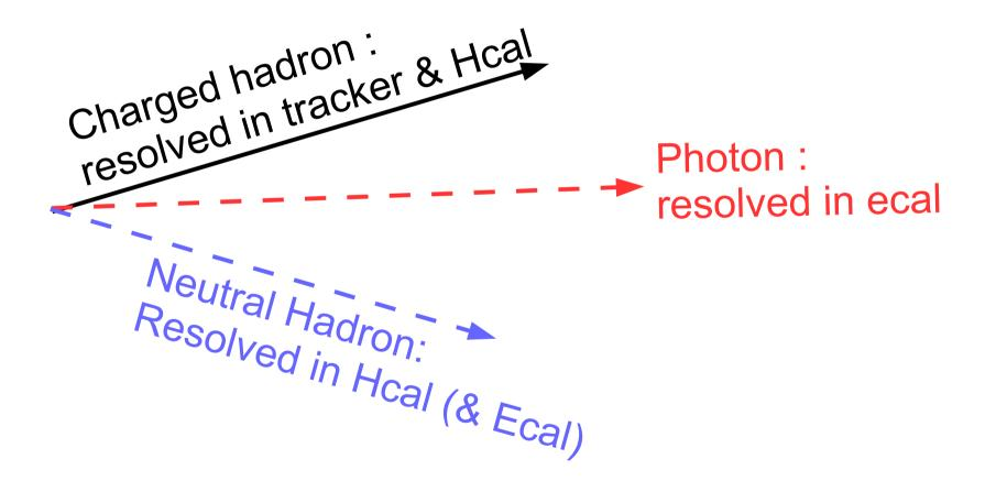
Key Question : What is the distance scale of each particle in the detector?
