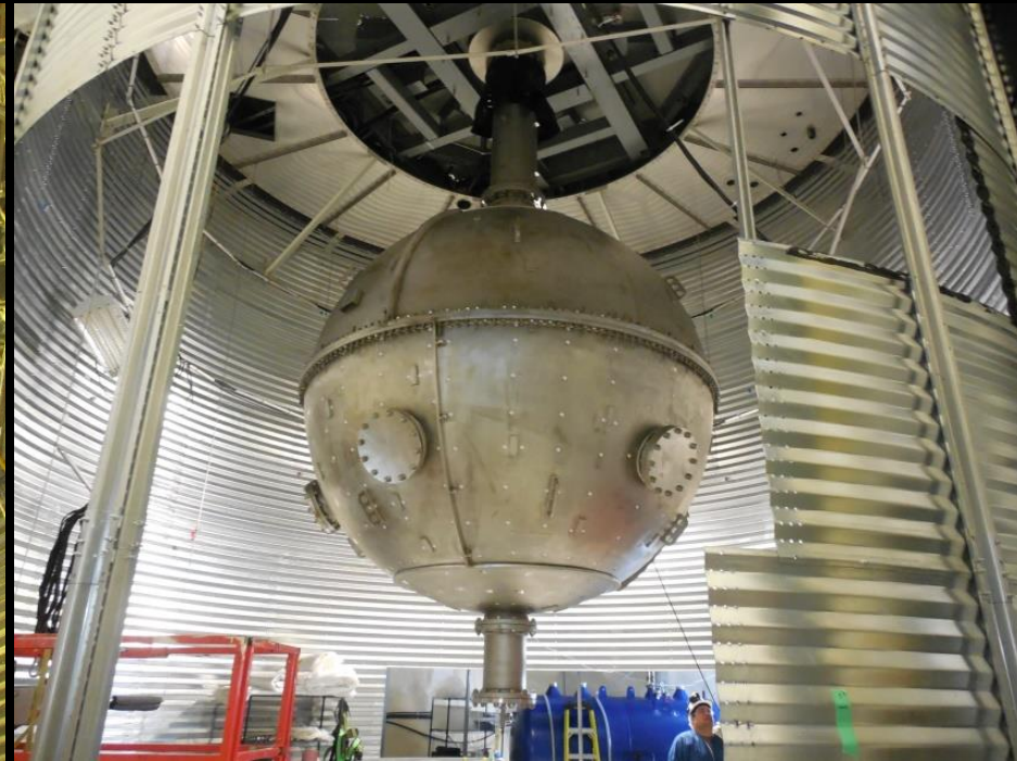
Steel Containment Sphere in 8m diameter water shield tank (water tank was filled Oct 2015)
